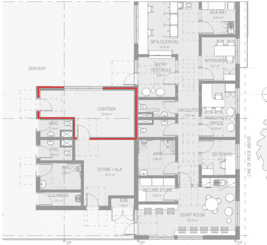
Figure 32: Canteen walls to have PIR insulation.
