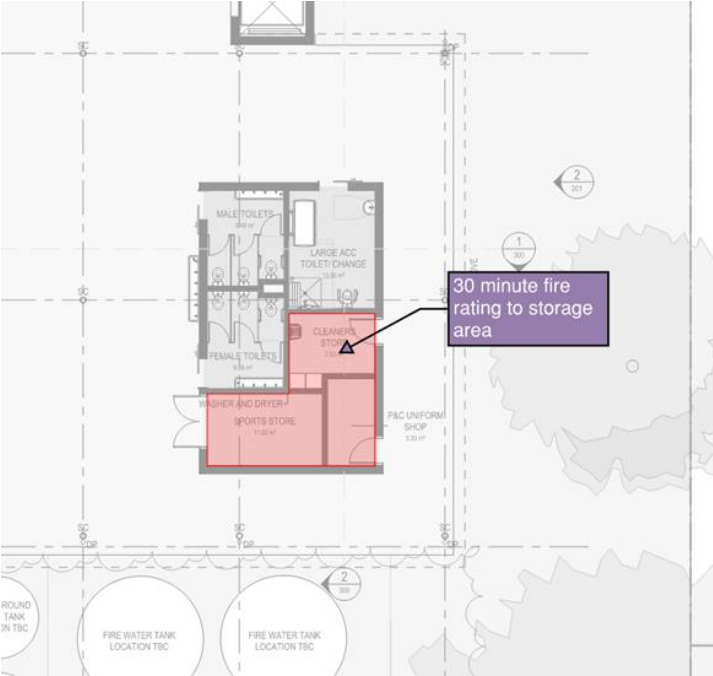
Figure 7: Storage area fire rating requirement
